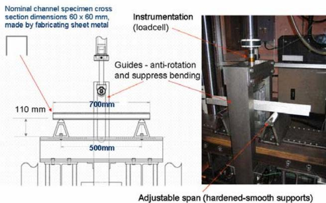
Figure 1: Bend-impact test arrangement: Specimen, fixture and boundary conditions
