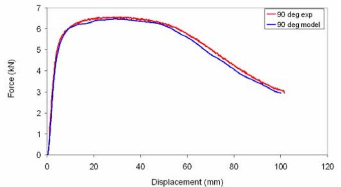
Figure 16: Aluminium alloy model correlation
