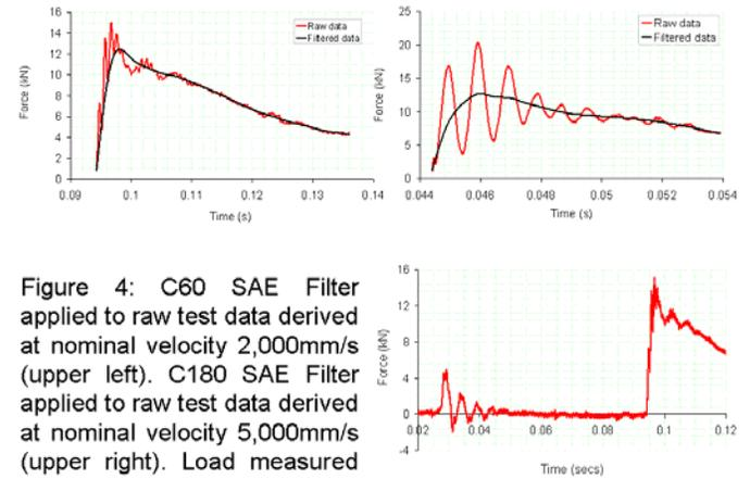
Figure 4: C60 SAE Filter applied to raw test data derived at nominal velocity 2,000mm/s (upper left). C180 SAE Filter applied to raw test data derived at nominal velocity 5,000mm/s (upper right). Load measured from transducer (lower)
