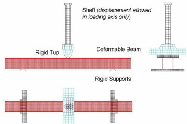
Figure 7: Model of experiment
