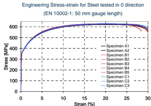
High accuracy and precision in deriving point properties such as yield point over the range of interest is expected from such smooth data. Such low variability could not be achieved when testing at high velocity in conventional high speed servo-hydraulic test machine systems due to a wider variety of error sources, promoting high variability and therefore increased error unless a large number of tests are conducted and this of itself leads to difficulty with interpretation, and incurs high cost.
