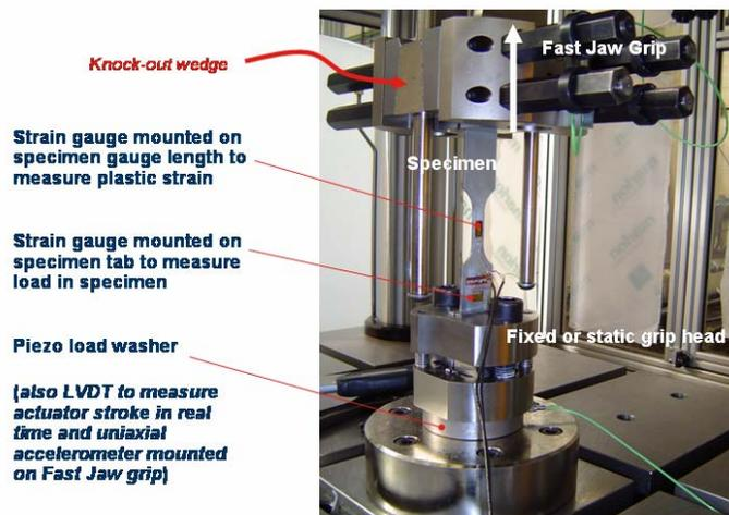
The principle of operation requires the fast jaw grip to be accelerated in the direction of the white arrow in figure 2 to reach target velocity. The knock out wedge is kicked out by a spacer rod pre-set by the test requirements, the grips are released to grab the specimen in typically  $5 \mu\text{s}$  ( $5 \times 10^{-6}$  sec).
