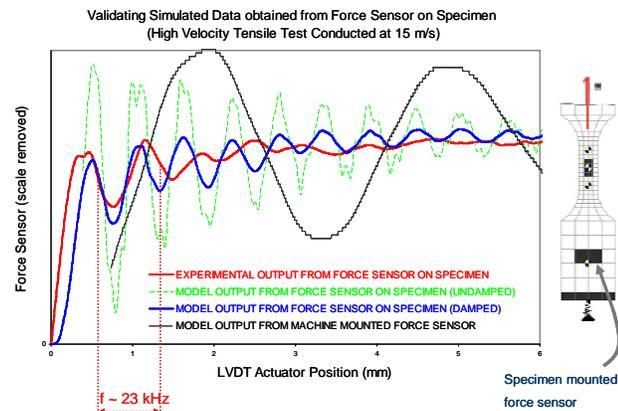
Figure 13: Frequency Response from Specimen Mounted Force Sensor
