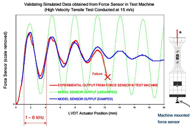
Figure 12: Frequency Response from Machine Mounted Force Sensor
