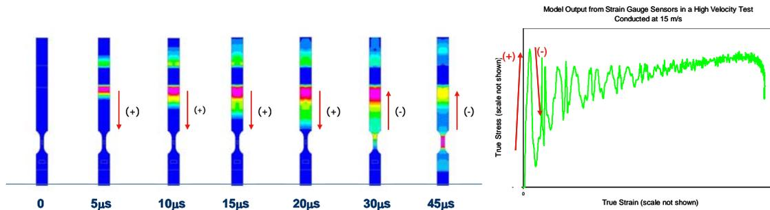
Figure 11: Movement of Stress Wave in Tensile Specimen on Load Take-up
