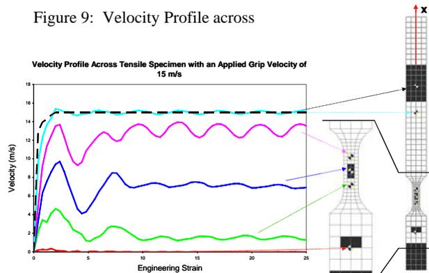
**System of Measurement – Strain Rate Measured from Strain Gauge Sensors in Model**
