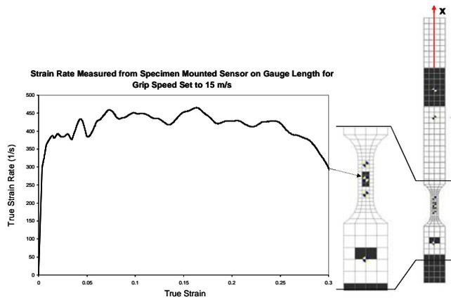
Figure 10: Strain Rate Measured from Specimen Mounted Sensor on Gauge Length
