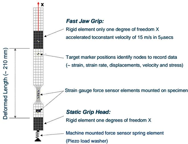
Figure 6: Model of Specimen, Sensors and Boundary Conditions
