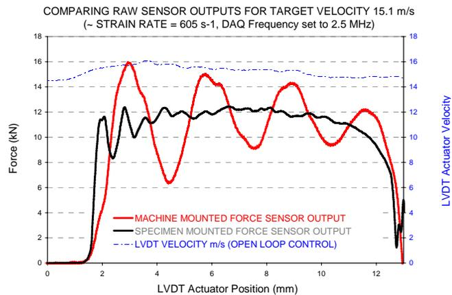
Figure 4: High Speed Test Data
