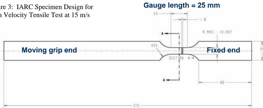
The conventional engineering strain rate is expressed by the formula grip velocity divided by initial gauge length<sup>[11]</sup>. The strain rate determined from this formula may be reasonable to a first approximation. The higher speed tensile specimen design shown has a gauge length of 25 mm, which may deliver a typical strain rate of  $600 \text{ s}^{-1}$  with an actuator velocity of 15 m/s. The short gauge length is expected to increase total elongation to failure.
