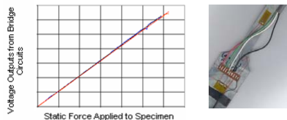
Figure 4. Quasi-static calibration curves
