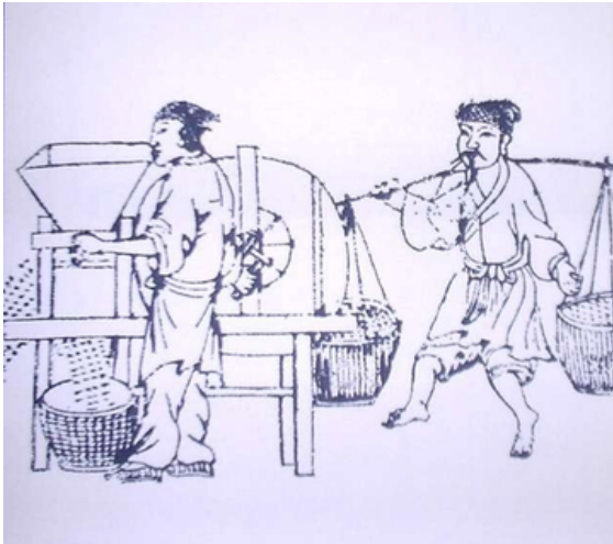
A winnowing machine illustration from Tiangong Kaiwu, one of Ming China's famous encyclopedias
