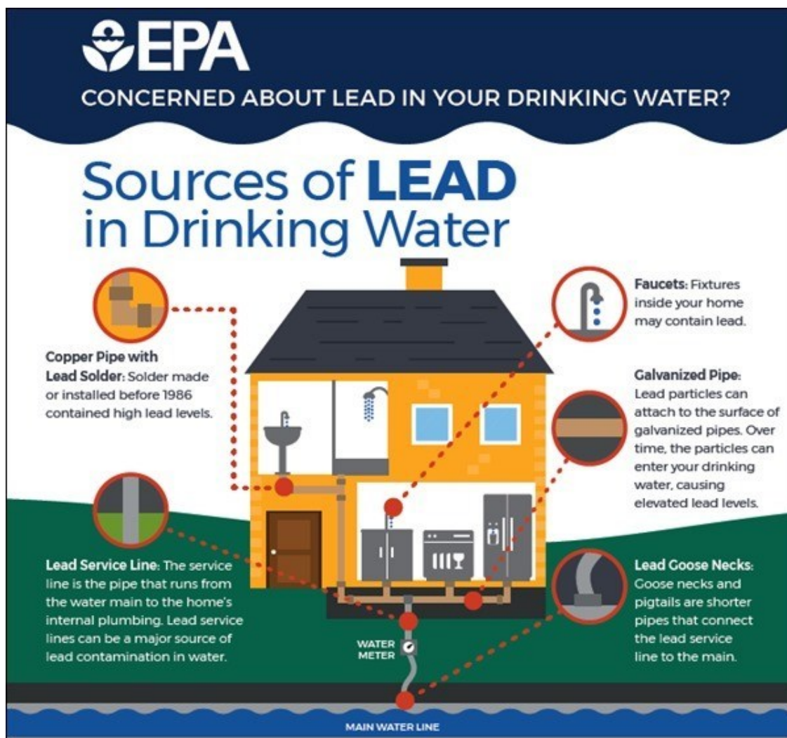
Figure A.2: Lead Pipes and Fixtures in the Home
