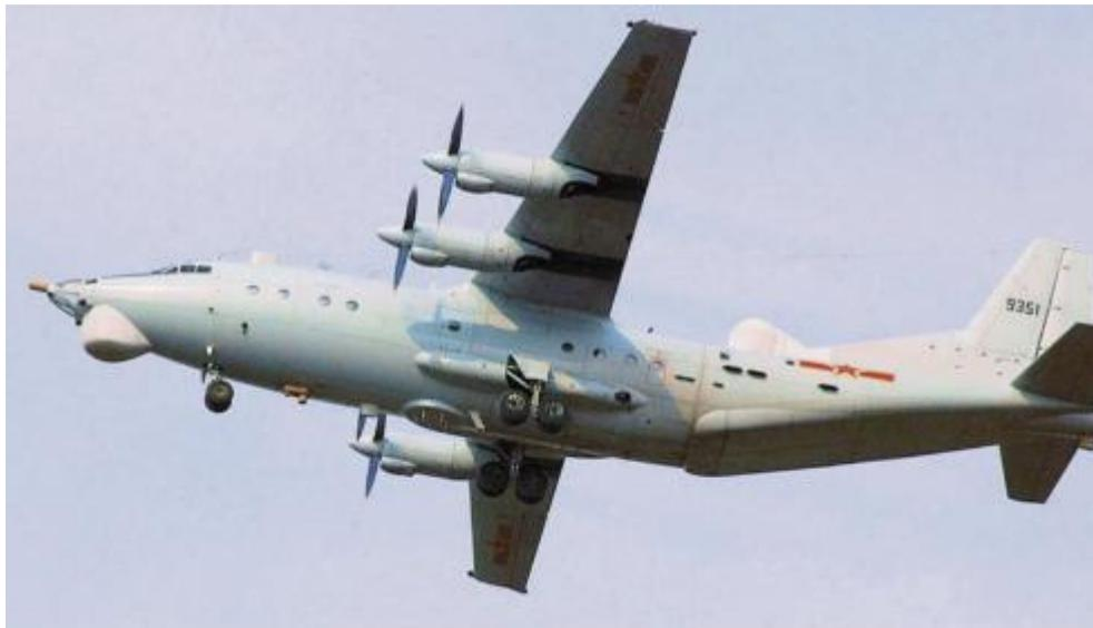
*Y-8(DZ) aircraft 9351 is one of a number of supposed SIGINT derivatives of China's Y-8 turboprop-powered transport aircraft. (Chinese Internet) 1299060*
