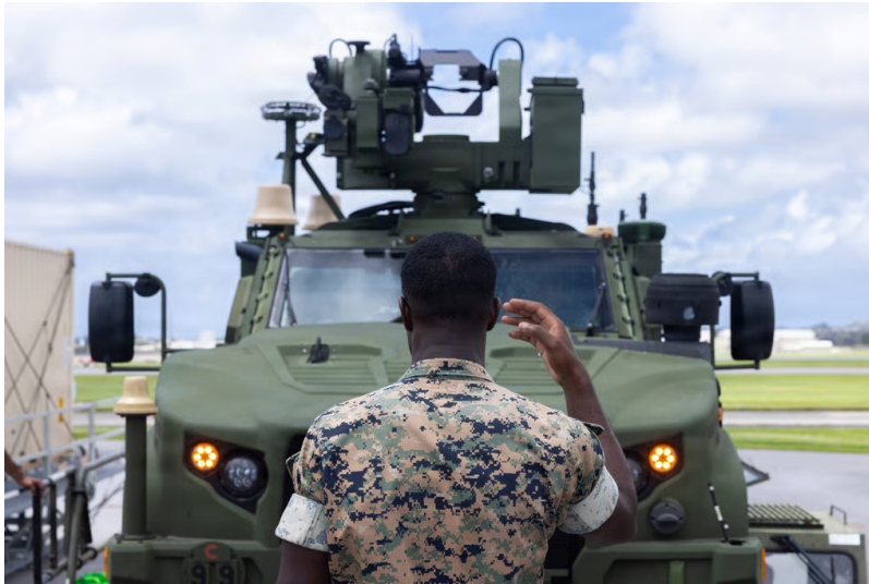
Madis is the US Marine Corps' advanced mobile air defence system designed to detect, track and neutralise drones and low-altitude aircraft using missiles, cannons and electronic warfare. Photo: Handout
