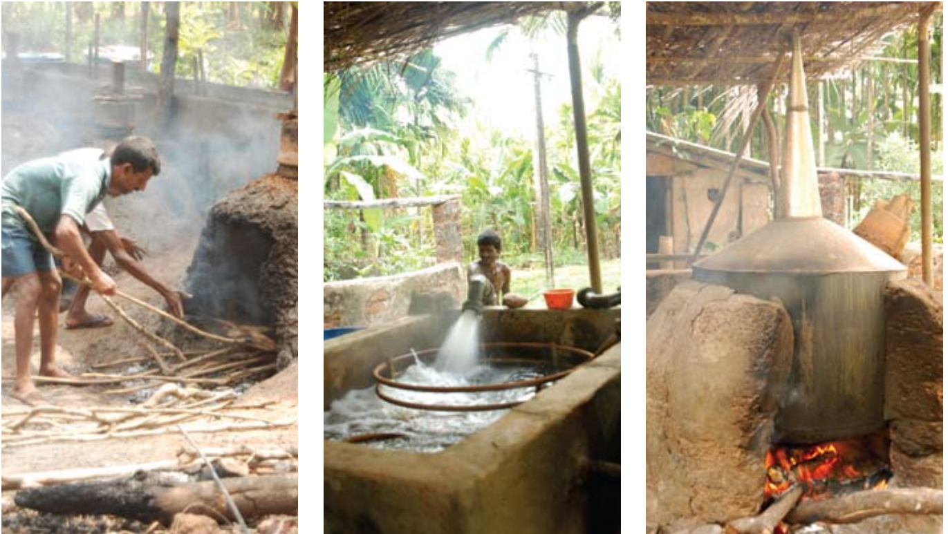
Photo 10: series of extralocal pot-still in operation (left) and a water tank with the coil being refilled (centre) and a large stainless steel pot-still at Sadashiv Marathe's distillery (right)
