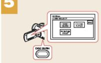
Press the DISC BURN button to start recording.
