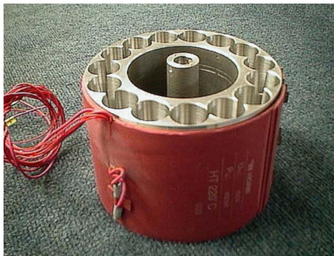
Figure 16 . Photograph of a 15-position vial oven taken from a TurboMatrix HS system. This has the capability to overlap the thermostating of up to 12 vials.
