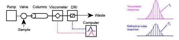
Using the universal calibration calculations are performed by the following methods:
