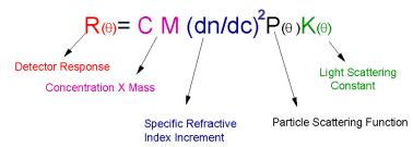
Where the particle scattering function is a measurement of the change in the relative intensity of light scattering as a function of angle.
