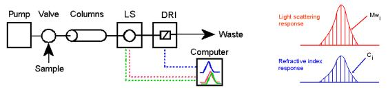
Using GPC Light Scattering calculations are performed by the following methods:
