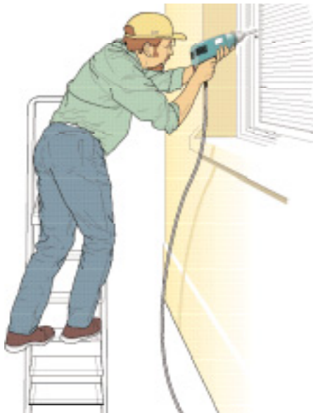
Figure 2a Incorrect - steps side-on to work activity
