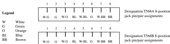
Eight-position jack pin assignments
