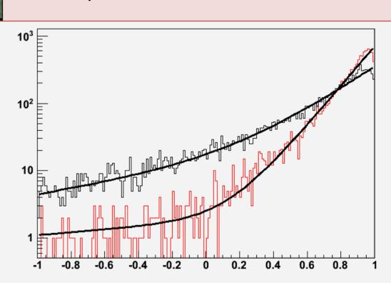
The  $\mu^+$  from  $\overline{\nu_{\mu}}$  is produced almost exclusively in the forward direction (cos $\theta$ >0). The results are from the GENIE Monte Carlo simulation. The histograms have been shown to be statistically inconsistent across the whole angular range, meaning charge separation will be possible
