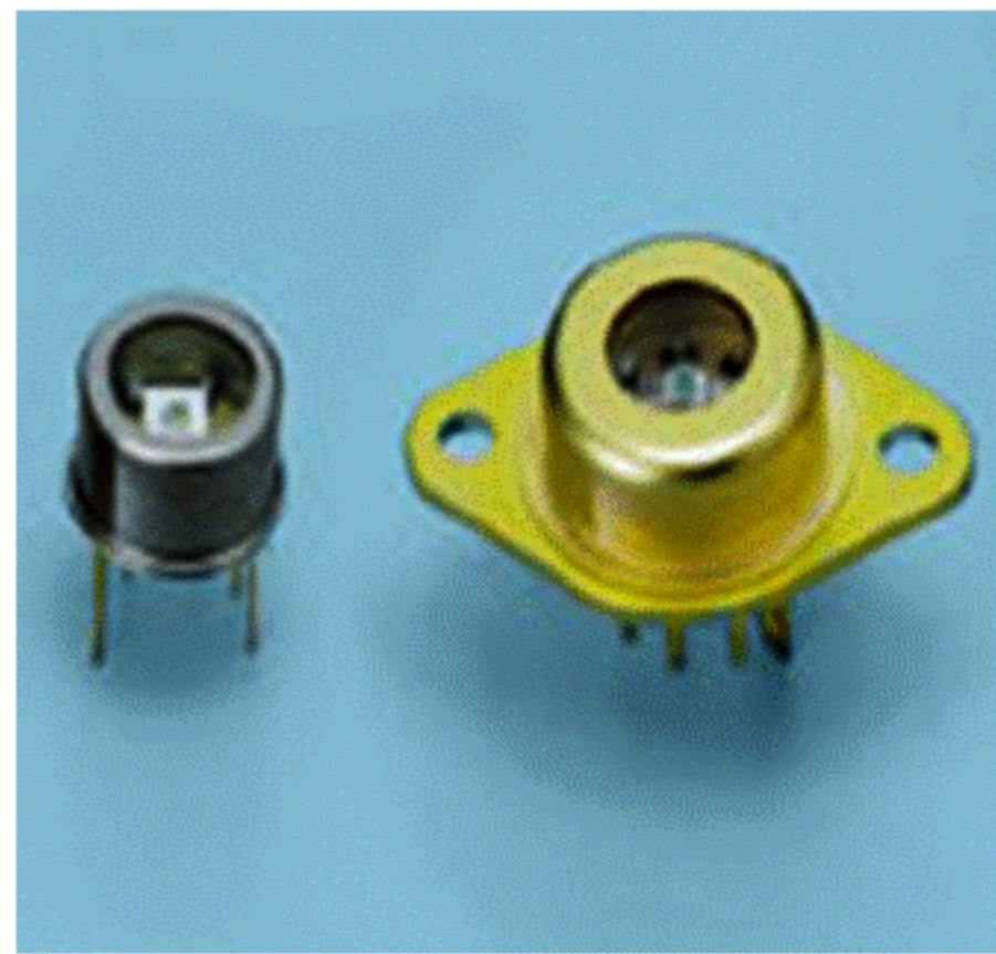
Two semiconductors, one Indium Antimonide (left) and the other Indium Arsenide (right). [1]
