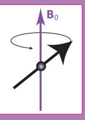
The sample is placed in a large magnetic field (B<sub>0</sub>), which nuclei precess around with a characteristic frequency,
