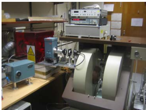
Figure 1. The EPR Spectrometer used throughout this investigation.
