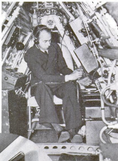
The flight engineer in his special compartment, surrounded by the 107 instruments and controls with which he keeps the engines working properly
