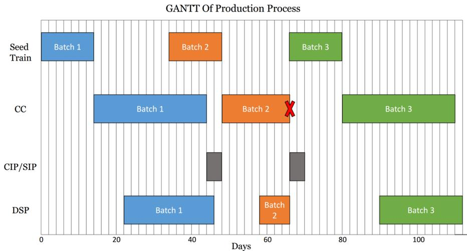
Figure: Mini GANTT of continuous process over three batches. CC = Cell Culture; CIP/SIP = Cleaning/Sterilisation-in-place; DSP = Downstream processing
