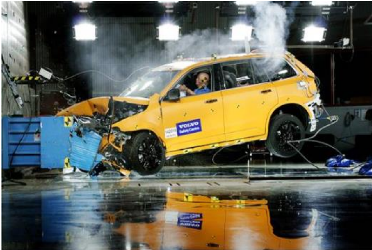
The Volvo XC90 undergoes a front offset crash test — Volvo
