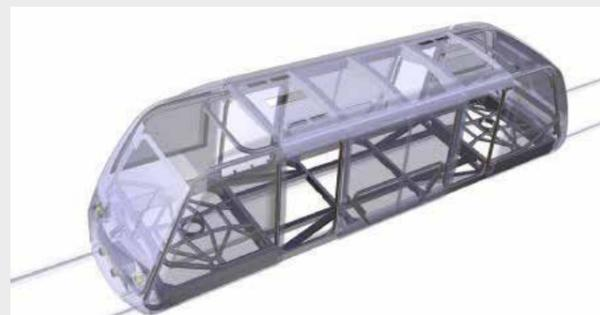
recycled or reused in other structures at its end of life. The reduced mass leads to a lower requirement for power and lowers the stress placed on the track system. This opens up significant cost saving opportunities in light rail systems. The technology ensures that the vehicle is tough for a long life in service, easily repairable and strong enough to protect the passengers on board.
