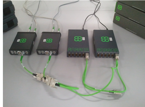
Fig. 1: Lab test setup for 4 ECUs.
